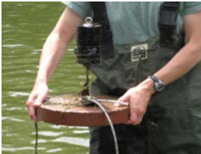
Hester-Dendy macroinvertebrate sampler and anchor stone used on the Fox River
